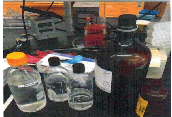
Figure 2: From left to right: Resolving Gel Buffer (1.5M Tris pH 8.8), Stacking Gel Buffer (1.0M Tris pH 6.8), 10% SDS, DDH2O, 30% Acrylamide.
